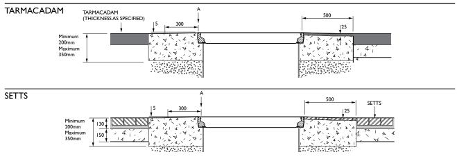
1.2m diameter solid base chamber with a corbel, adjustable skirt, non-structural internal lid and round 900mm flat sealed cover with central manual dip cover. Round Tank Flange.
