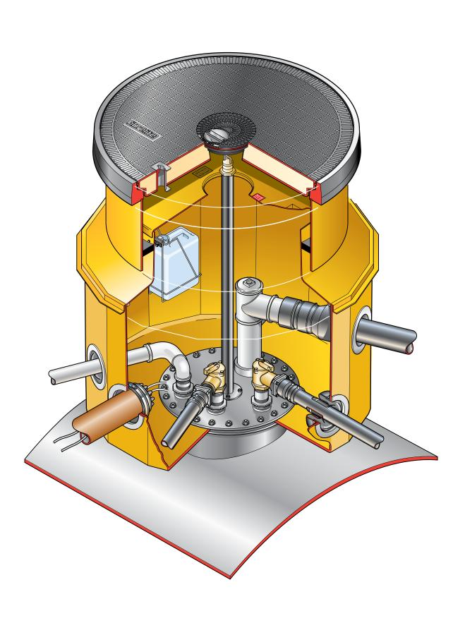
1.2m diameter solid base chamber with a corbel, adjustable skirt, non-structural internal lid and round 900mm flat sealed cover with central manual dip cover. Round Tank Flange.
