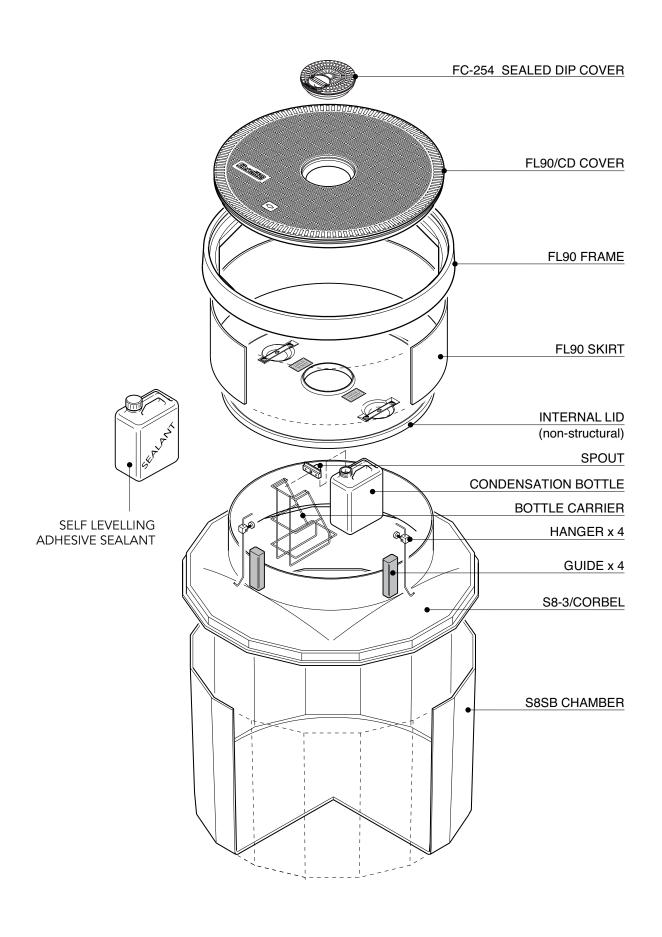
1.2m diameter solid base chamber with a corbel, adjustable skirt, non-structural internal lid and round 900mm flat sealed cover with central manual dip cover. Round Tank Flange.
