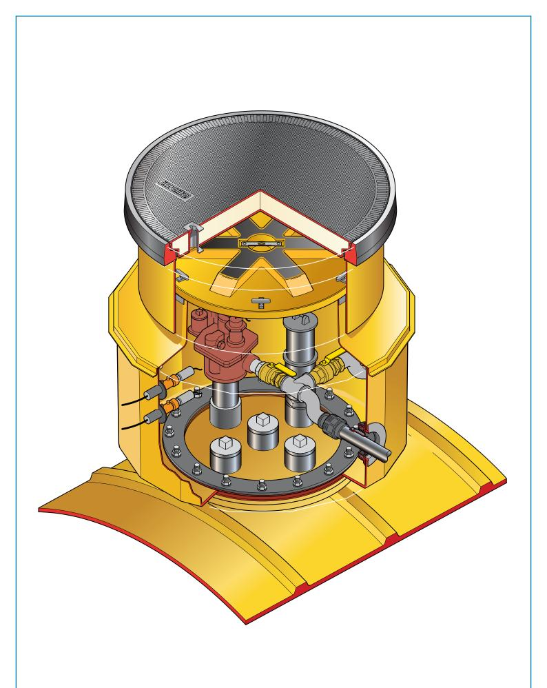
1.2m diameter solid base chamber with a sealed corbel, watertight platform, adjustable skirt, and round 900mm flat sealed cover.
