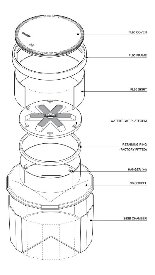
1.2m diameter solid base chamber with a sealed corbel, watertight platform, adjustable skirt, and round 900mm flat sealed cover.
