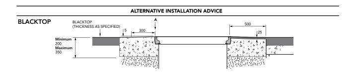
1.2m diameter solid base chamber with a sealed corbel, watertight platform, adjustable skirt, and round 900mm flat sealed cover.
