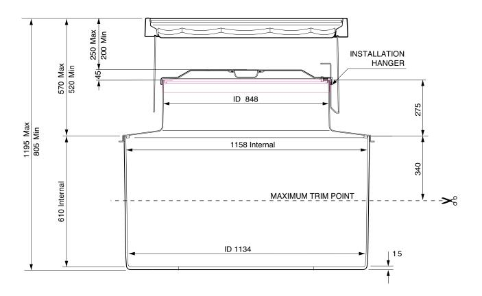
1.2m diameter solid base chamber with a sealed corbel, watertight platform, adjustable skirt, and round 900mm flat sealed cover.
