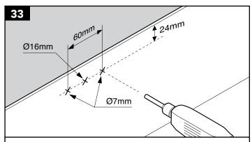
Mark out the position of 2 No. holes to be drilled 24mm down from the top edge of the corbel and 60mm cross centre. Drill the two Ø7mm holes into the Corbel walls.
