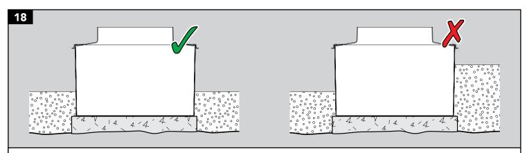
Carefully backfill the area around the sump with peagravel or sand. Backfill equally around the sump in layers to prevent damage or deformation.
