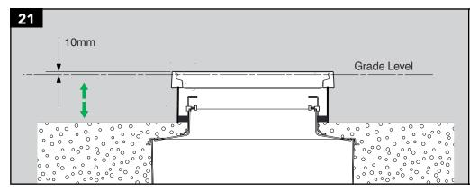
Adjust knobs to set the frame to stringline level, adjust for fall in grade. Set the frame 10mm above grade level.
