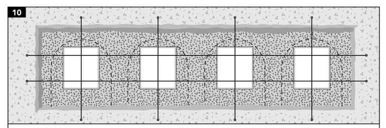
Fix string lines 10mm above grade level across the length and width of the sump to highlight any falls. When backfilling ensure the pipework is not disturbed.
