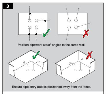
**WARNING** Care must be taken to position the pipework and conduit so it exits the sump at 90° angle to the sump wall. Otherwise undue stress will be placed on the sump wall and entry boot, which may lead to leaks in the future.
