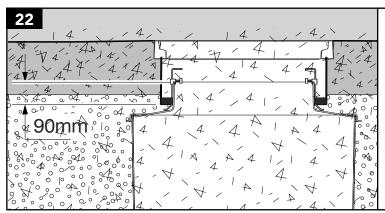
Ensure the void between corbel and skirt is kept free from concrete and a depth of 90mm overlap minimum is maintained.
