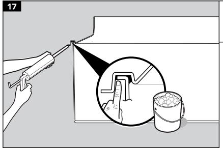
Seal around the outside joint and smooth off sealant with soapy water.
