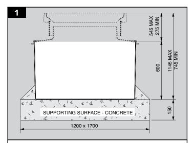
Position the sump onto an adequate supporting surface to the correct height.
