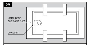
Drain and bottle should be positioned away from pipe risers and STP. The drain must be installed at the created low point to do this. Compact the sand in a way to create a low point 10-15mm lower than the surrounding sand.
