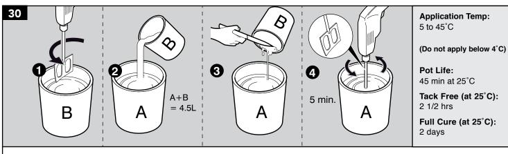
Using a suitable container stir the contents of Pack B and add the entire contents to Pack A to give a combined content of 4.5Ltrs. Ensure white sediment from can B is put into can A before mixing. Stir for a full 5 minutes using a slow speed electric drill (400 - 500 RPM) with a mixer paddle until a completely homogeneous mix is obtained. Take care to avoid including excess air. Mixing is made easier if the Pack B is added and mixed in two stages.
