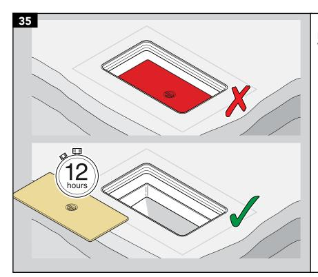
Do not install the internal lid until the sealant has set. Wait overnight
