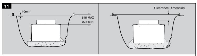
Place the corbel onto the sump (only 'dry fit' the corbel do not bond at this stage). Check the measurement from the top of the corbel to the string line, which is set 10mm above the general grade level. Check all sides of the sump and select the largest and smallest measurement to take account of falls across the forecourt.
