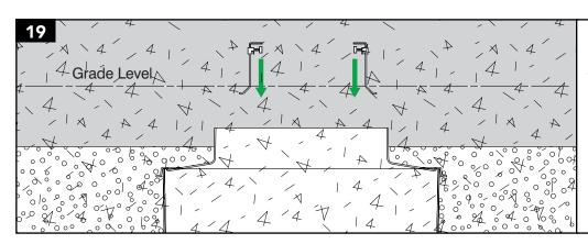
Fix a string line 10mm above grade level across the sump, fix 4 hangers on the corbel top with base support facing out.
