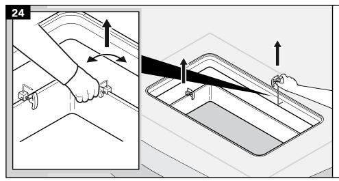
After minimum concrete cure time, hangers can be removed. Loosen the 'T' knob, push down on the rod, turn the rod through 90° and pull rod up to remove.
