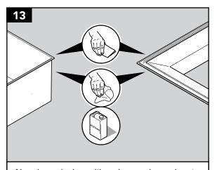
Abrade and wipe with a degreasing solvent the chamber or extension top edge/wall and the corbel groove.
