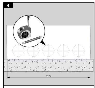
Mark out the required number of pipes in the sump.
