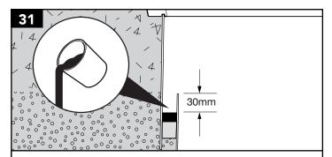
1 set of cans A+B will seal 2 sumps. Decant mixture from can A into can B to have more control when pouring the mixture into the void, onto the sand base. Avoid spilling the contents to ensure a clean finish on the side walls of corbel and skirt. The sealant shall be poured to level 30mm below the top edge of the Corbel (the amount of sealant required is dependant on the height of the system but should be between 1.5 and 1.7 Litres).
