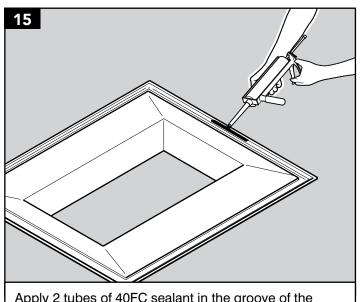
Apply 2 tubes of 40FC sealant in the groove of the corbel. Sealant should fill half the groove.
