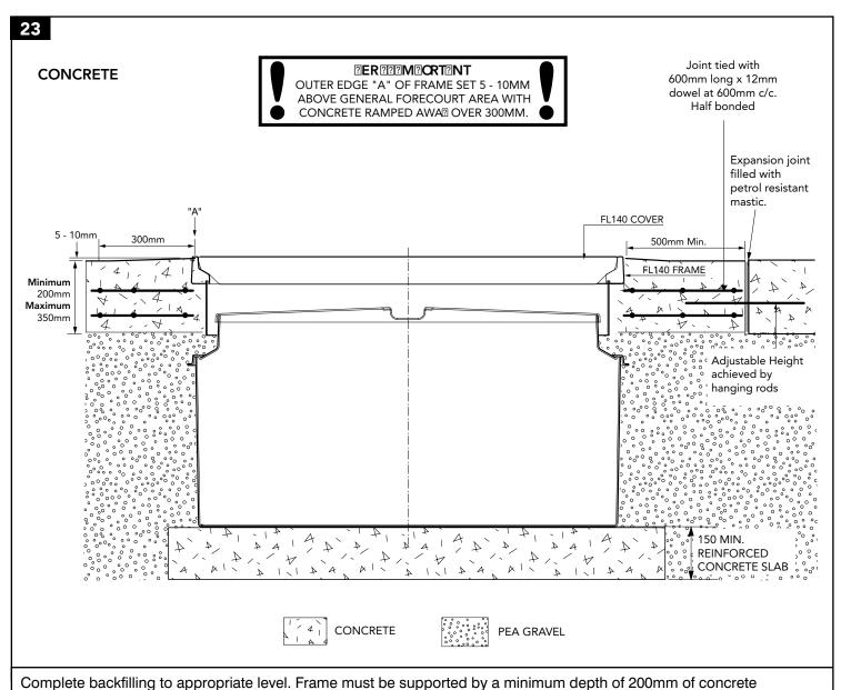
Concrete ties must be inserted as close to the frame as possible. Minimum block of 500mm square around the frame.
