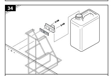
Ensure the rubber gasket is fitted to the mating surface of the bottle hanger. Secure the Bottle Hanger to the Corbel wall with 2 No. M6 x 15 Dome Head Screws and Washers.
