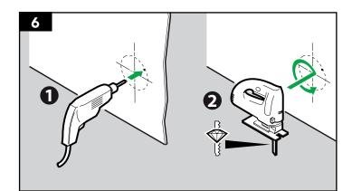
For larger holes (190mm) we recommend that the hole is marked and jigsaw is used to cut the hole. Firstly, drill a hole through the wall, so the jigsaw can be inserted and used easily and safely.
