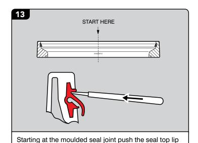
into the extrusion seal housing by running the blade
