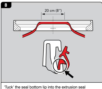
'Tuck' the seal bottom lip into the extrusion seal housing for approximately 20 cm (8")
