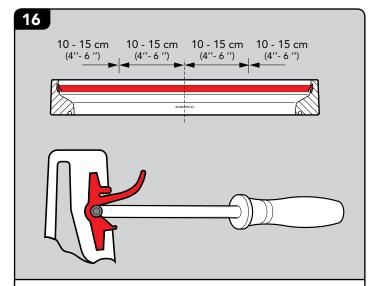
Put the fitting tool onto the nylon tube and run the tube into position whilst holding the main seal open. Perform this operation in stages of 10-15 cm (4"-6").
