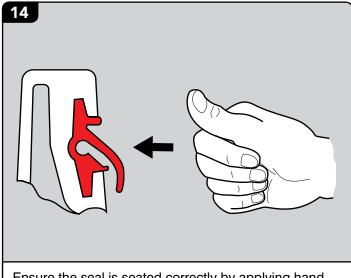
Ensure the seal is seated correctly by applying hand pressure to the front face of the seal.
