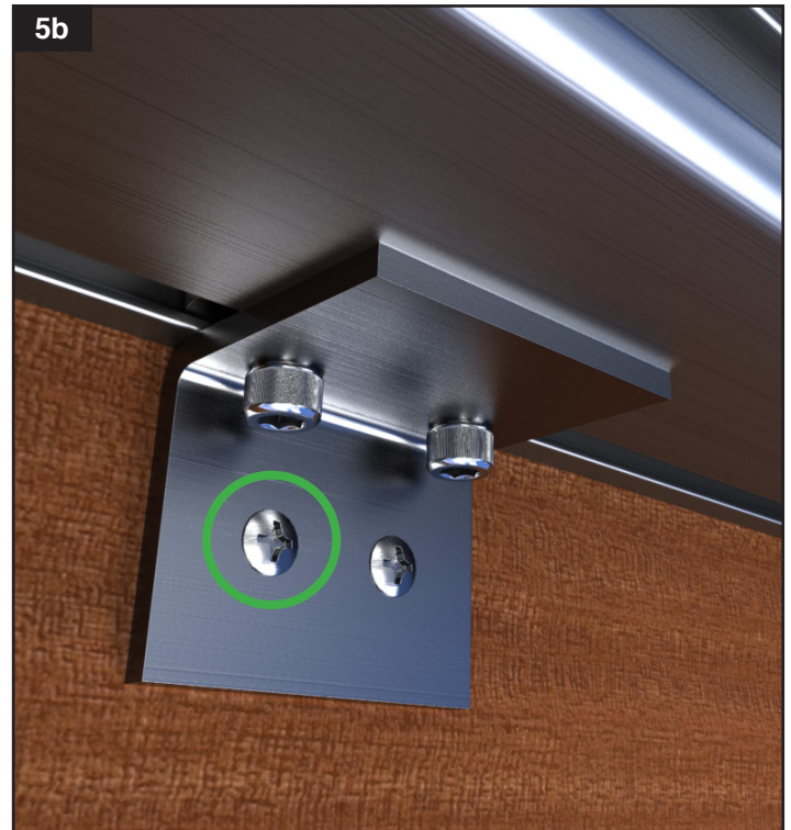
Using screws (#12 wood screw) or nails (10d to 60d), fix the frames with hangers to the exterior of the wood trench form.
