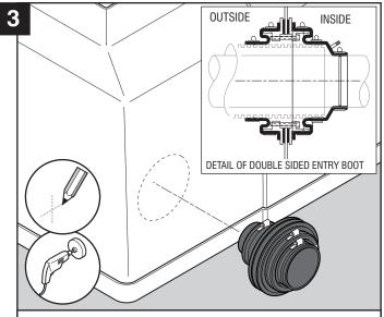
If Fibrelite penetration fittings are to be used (PSB 50 to 110, PSBD 50 to 110 and PDBD pipe entry kit models a  $\varnothing$  6" hole should be drilled). Mark up the hole positions.
