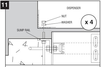
Remove upper nut & washer on the 4 anchor bolts Install & connect the dispenser to the sump frame & anchor bolt. Fit & tighten nut & washer.
