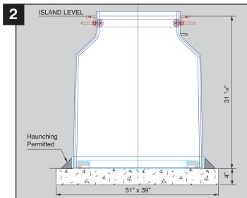
Dry fit the sump to ensure it sits level and prepare an adequate support base.
