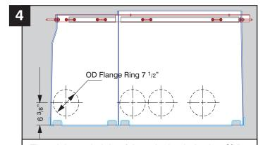
The minimum height of the exit pipe holes is 6 3/8" from the sump base to the holes centreline.
