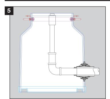
Run pipework through side wall, connect to upward riser.
