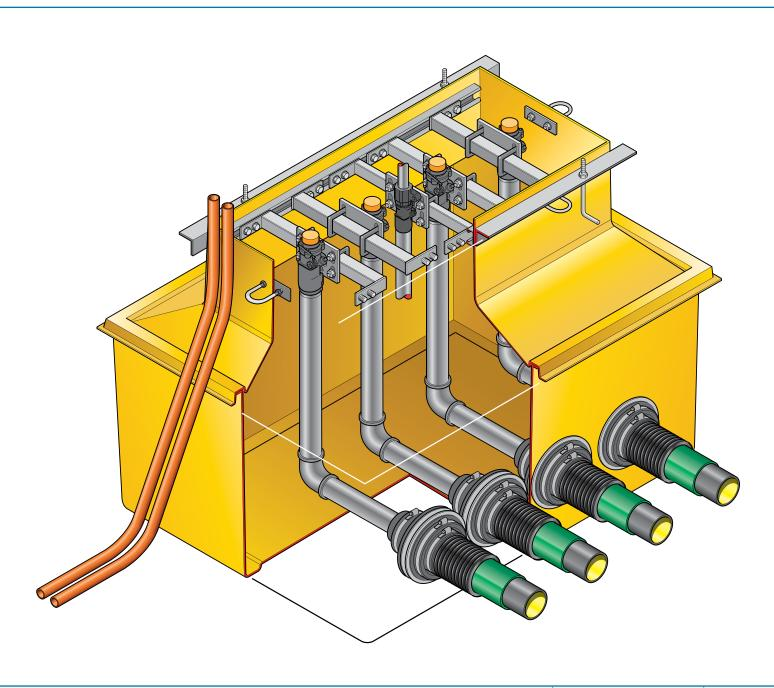
43" x 32" FRP solid base sump and corbel to fit Gillbarco dispenser model Encore 500. 4 Product. Includes dispenser support rails, shear valve rails and all fixings. Metalwork reference SIM322.
