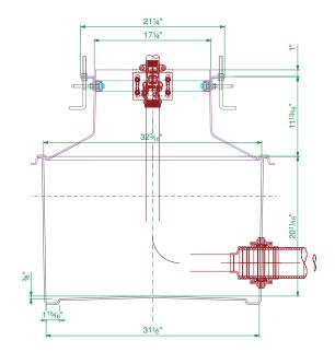
43" x 32" FRP solid base sump and corbel to fit Gillbarco dispenser model Encore 500. 4 Product. Includes dispenser support rails, shear valve rails and all fixings. Metalwork reference SIM322.
