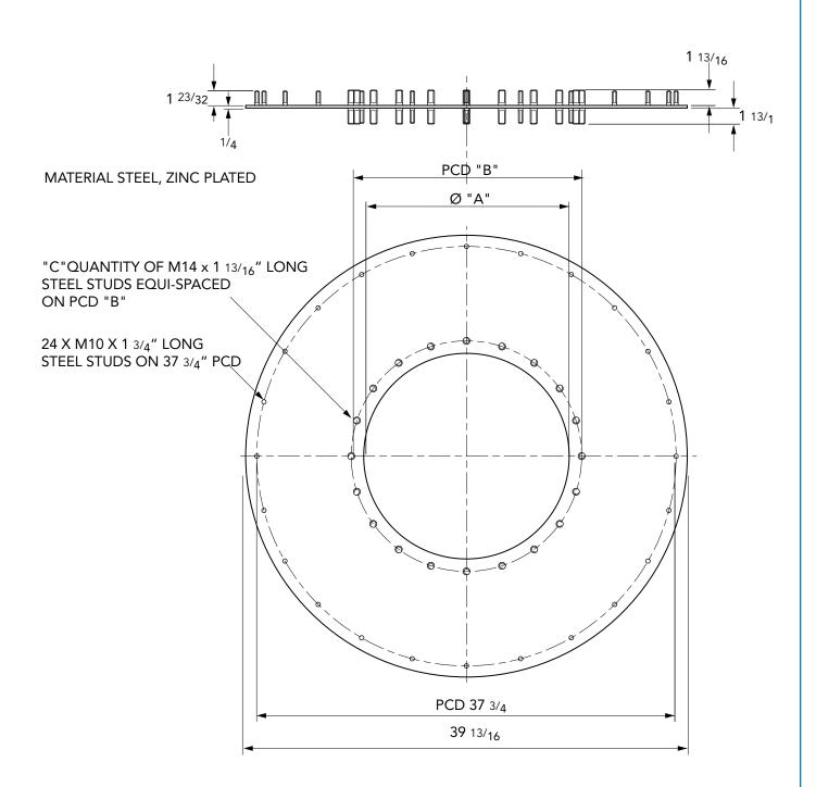
DIMENSIONS A, B & C TO BE DETERMINED BY SPECIFIC INSTALLATION
