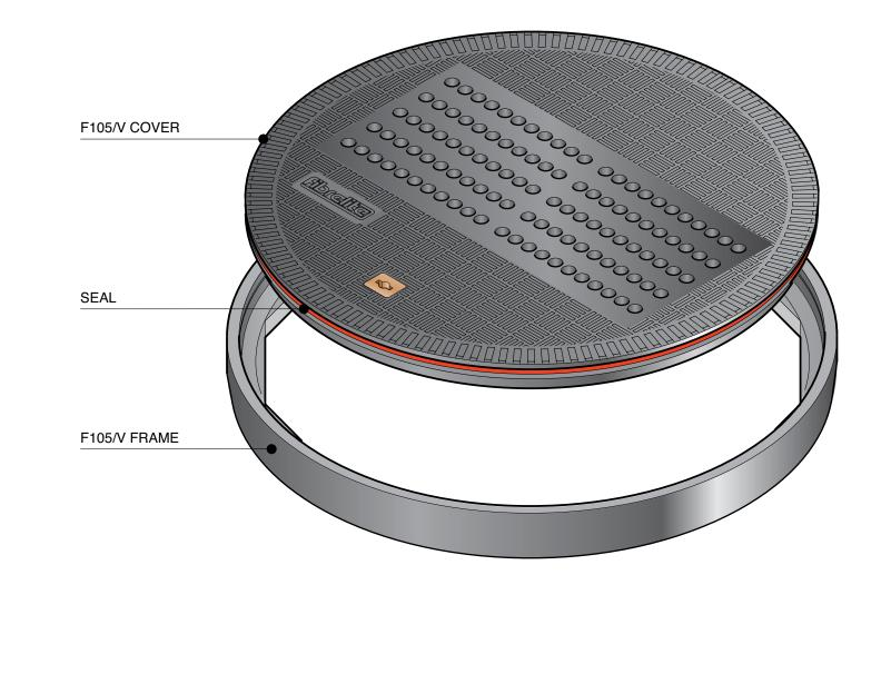
40° diameter vented, flat cover with composite frame. Temperature & chemical resistant. Designed for steam applications. For reference purposes only. This drawing is not a specification. Order against product code only. To enable continuous improvement of our products, the designs and specifications are subject to change without notice. F105-V Issue: 11/06/2016
