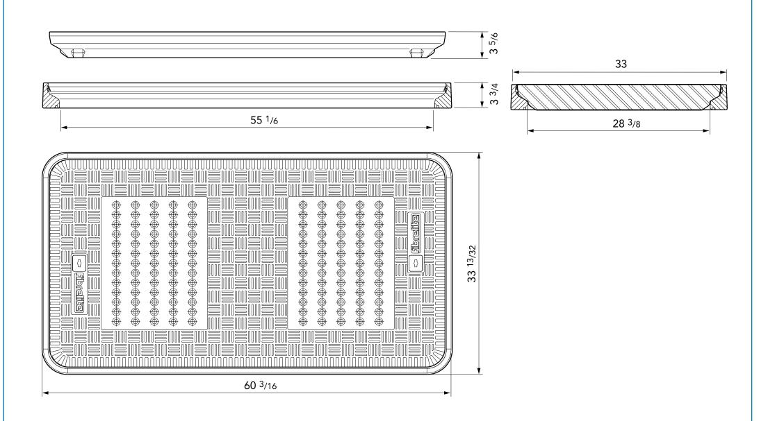
55" x 28" flat vented, composite cover with aluminum frame. Temperature and chemical resistant. Designed for steam applications.
