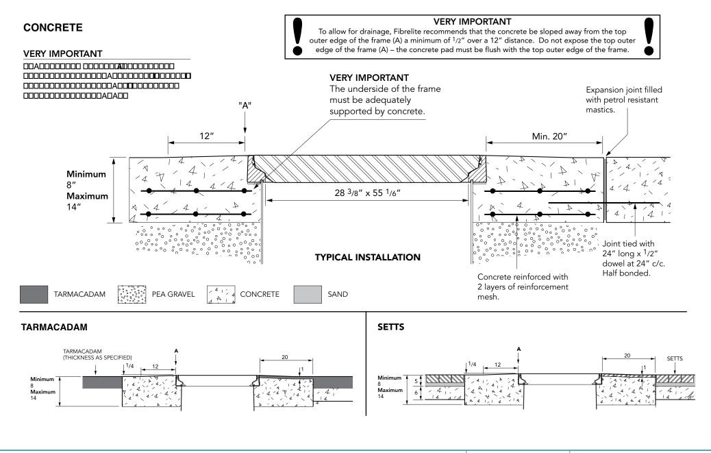
55" x 28" flat vented, composite cover with aluminum frame. Temperature and chemical resistant. Designed for steam applications.
