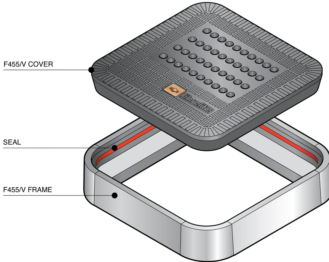
18" x 18" square vented, flat composite cover with aluminum frame. Temperature & chemical resistant. Designed for steam applications.
