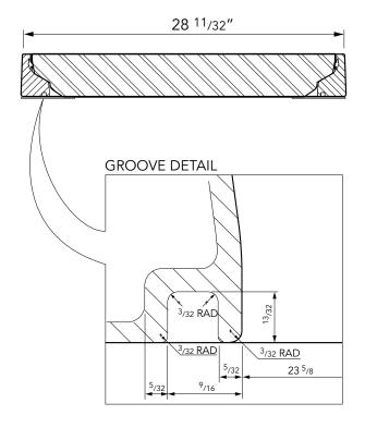
24" x 24" flat, vented composite cover with an aluminum frame. Temperature & chemical resistant. Designed for steam applications.
