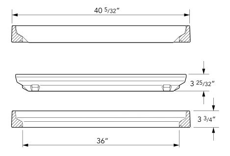
36"square vented, flat composite cover with an aluminum frame. Temperature & chemical resistant. Designed for steam applications.
