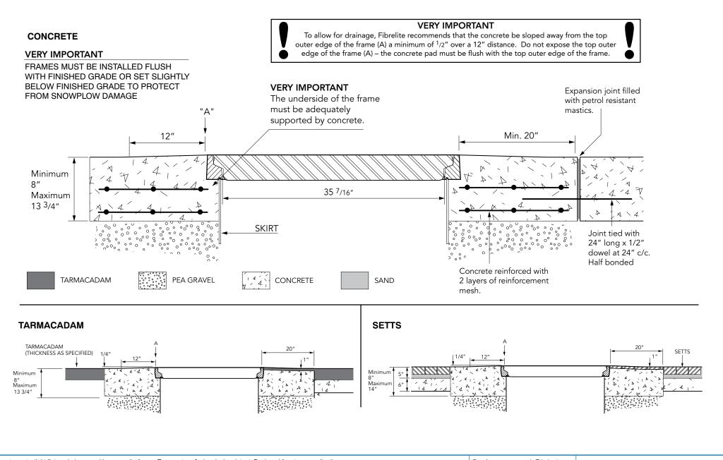
36" diameter watertight flat sealed cover with composite frame. Temperature & chemical resistant. Designed for steam applications.
