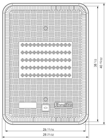
36" x 24" flat, vented composite cover with aluminum frame. Temperature and chemical resistant. Designed for steam applications.
