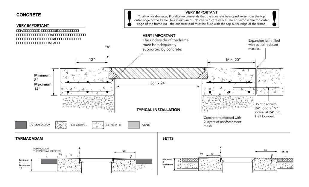
36" x 24" flat, vented composite cover with aluminum frame. Temperature and chemical resistant. Designed for steam applications.
