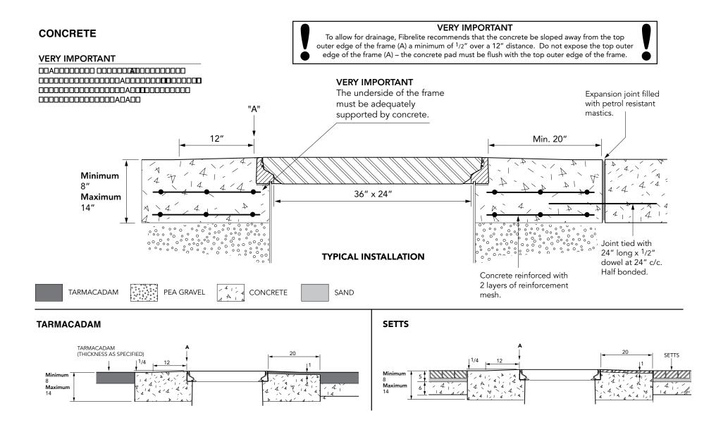
36" x 24" flat sealed composite cover with aluminum frame. Temperature and chemical resistant. Designed for steam applications.
