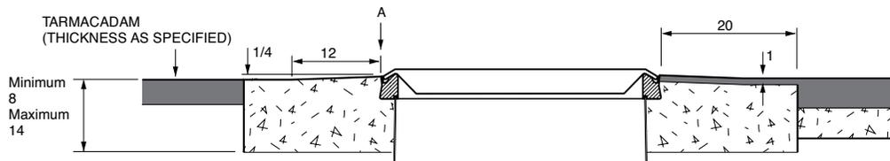
30" x 30" raised composite cover with an aluminium frame.
