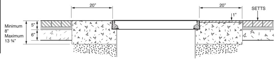
40" diameter flat sealed composite cover and frame.
