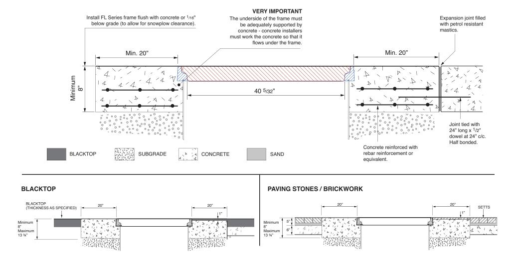
40" diameter flat sealed composite cover and frame.
