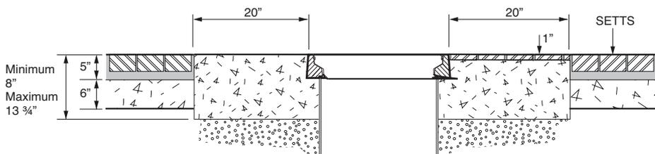
12" diameter flat sealed composite cover and frame.
