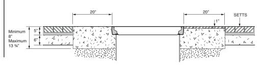
55" x 28" flat sealed composite cover with an aluminum frame.
