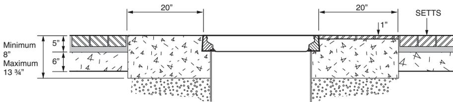
18" diameter flat sealed composite cover and frame.
