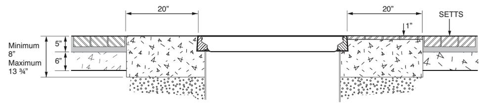
24" diameter flat sealed composite cover and frame.
