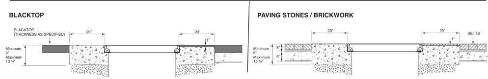
24" diameter flat sealed composite cover and frame.
