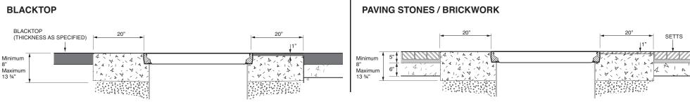
30" x 30" flat sealed composite cover with an aluminum frame.
