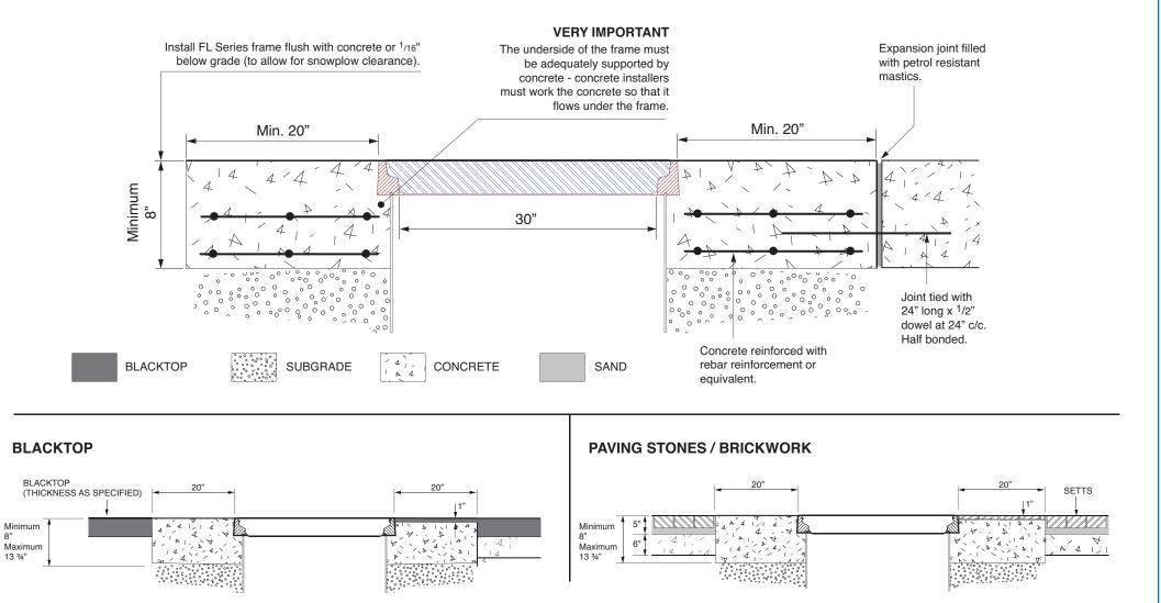
30" diameter flat sealed composite cover and frame.
