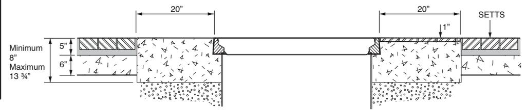
36" diameter flat sealed composite cover with a composite frame.
