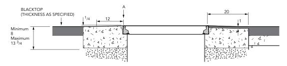
36" diameter flat sealed composite cover with conposite frame.
