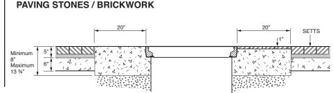
36" x 24" flat sealed composite cover with an aluminum frame.
