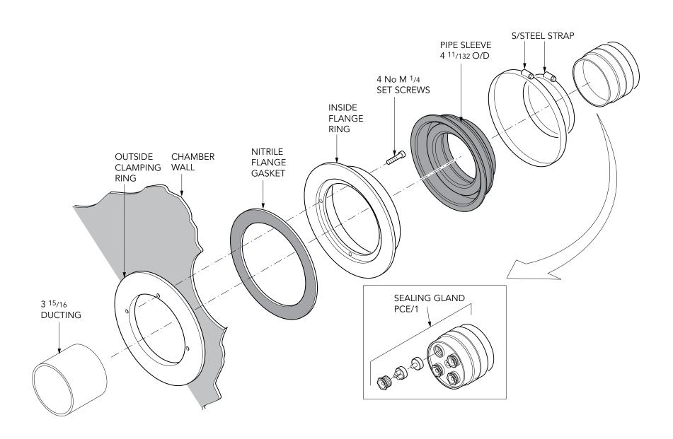
411/32" dia. pipe entry seal kit (PSB/110), with sealtight compression gland. Sealing gland fits 4 cables (11/32" - 25/32") or 12 cables (5/32"-5/16"). Internal sealing gland can be purchased separately. (PCE/1)
