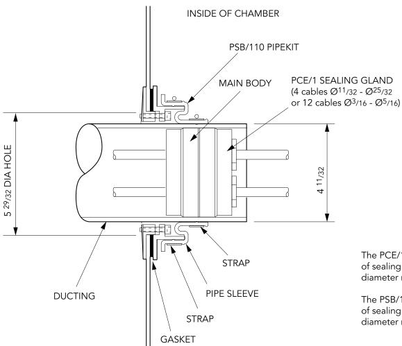
The PCE/1 sealing body is capable of sealing to ducts with an internal diameter ranging from 3 <sup>13</sup>/<sub>16</sub> to 4 <sup>11</sup>/<sub>32</sub>.
