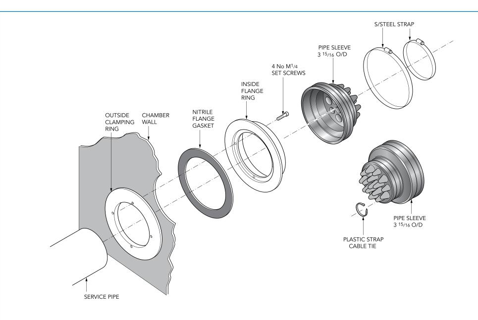
4 11/32 dia. rubber cable entry kit designed to seal up to 16 cables. Supplied with cable ties.
