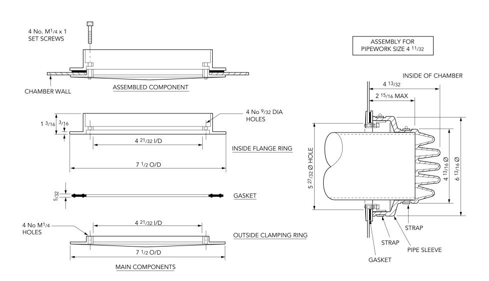
4 11/32 dia. rubber cable entry kit designed to seal up to 16 cables. Supplied with cable ties.
