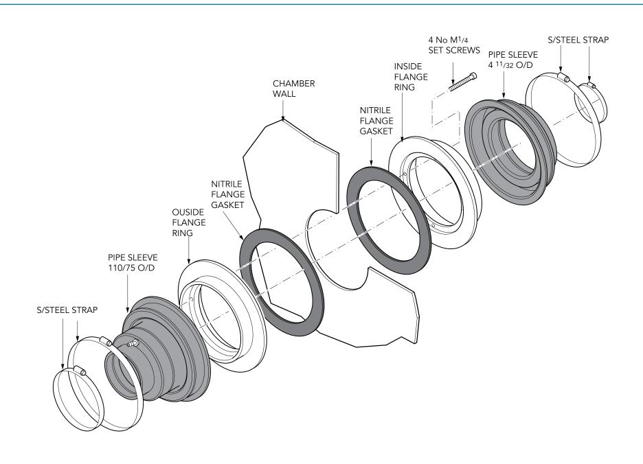
Dual Bore Pipe Entry kit suitable for 4 11/32" - 2 15/16" Pipe.
