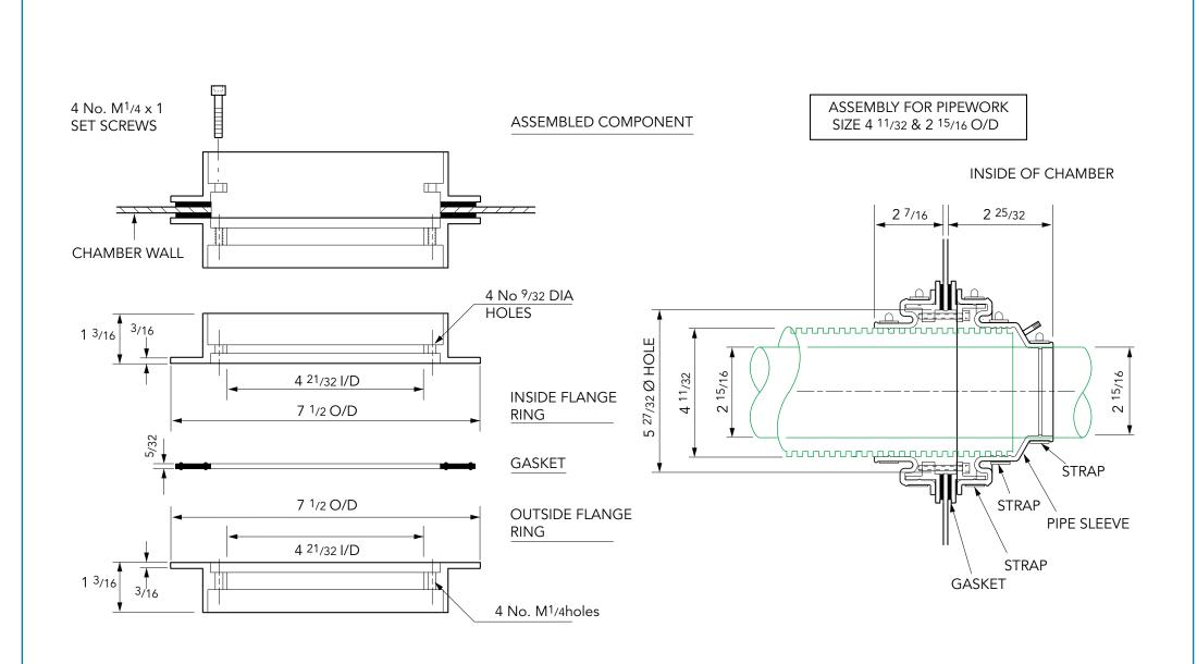
Dual Bore Pipe Entry kit suitable for 4 11/32" - 2 15/16" Pipe.
