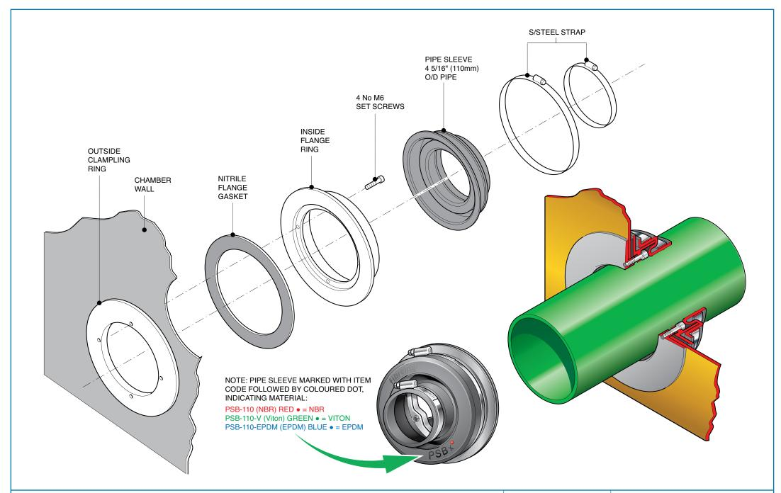
Pipe entry kit to fit 4 5/16" (110mm) single bore pipework.
