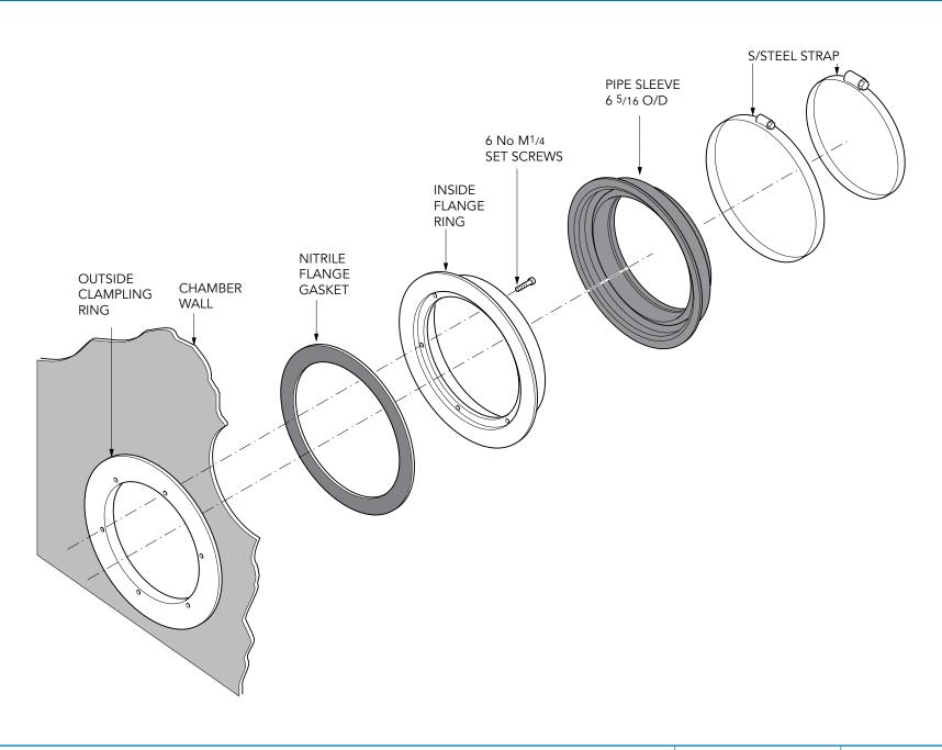
Large clearance pipe entry kit to 6 5/16" pipe.
