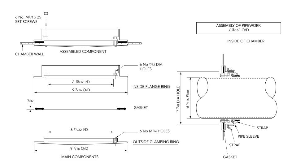
Large clearance pipe entry kit to 6 5/16" pipe.
