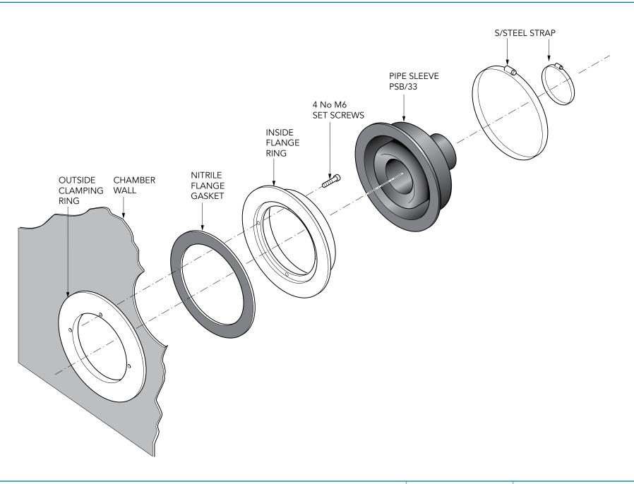
Pipe entry kits to fit 1" steel conduit.
