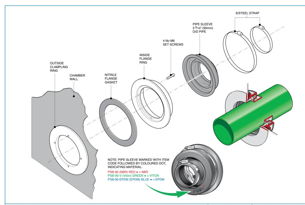
Pipe entry kit to fit 3 9/16" (90mm) single bore pipework.
