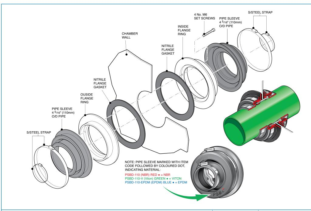
Double sided pipe entry kit to fit 4 5/16" (110mm) single bore pipework.
