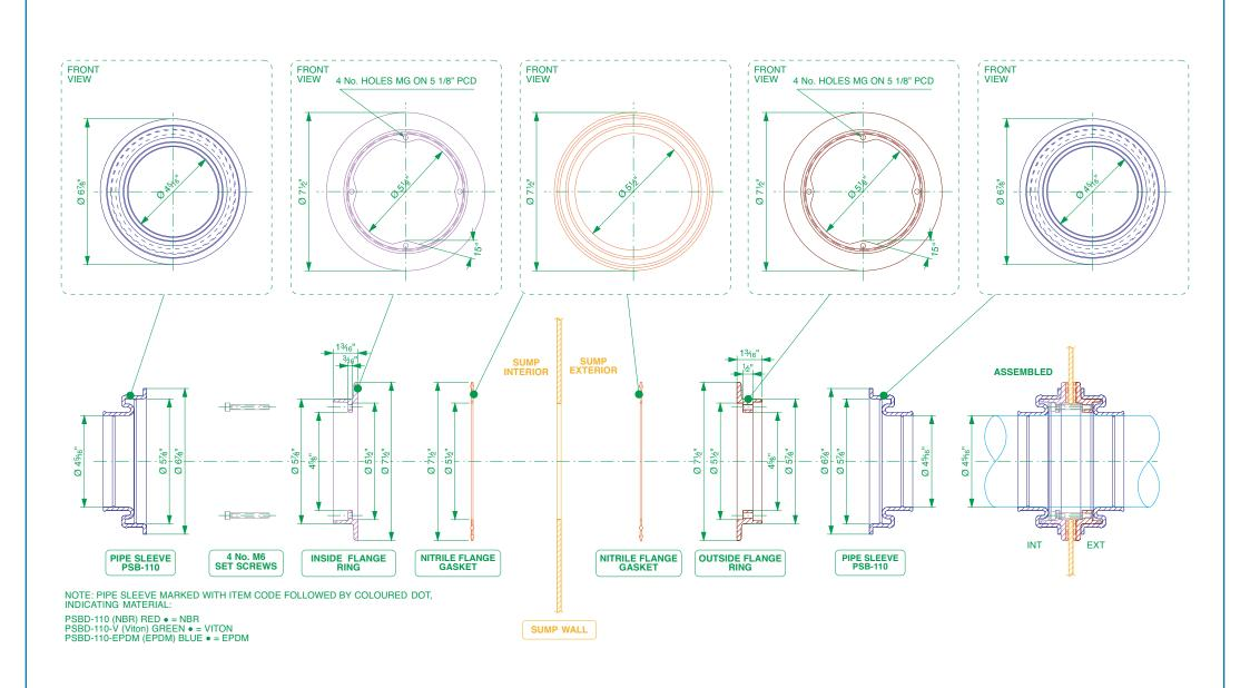
Double sided pipe entry kit to fit 4 5/16" (110mm) single bore pipework.
