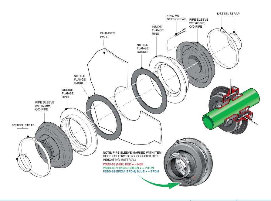
Double sided pipe entry kit to fit 2 1/2" (63mm) single bore pipework.
