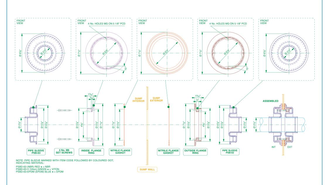
Double sided pipe entry kit to fit 2 1/2" (63mm) single bore pipework.
