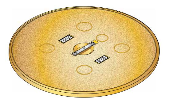
Hole configuration used for offset manual dipping.
