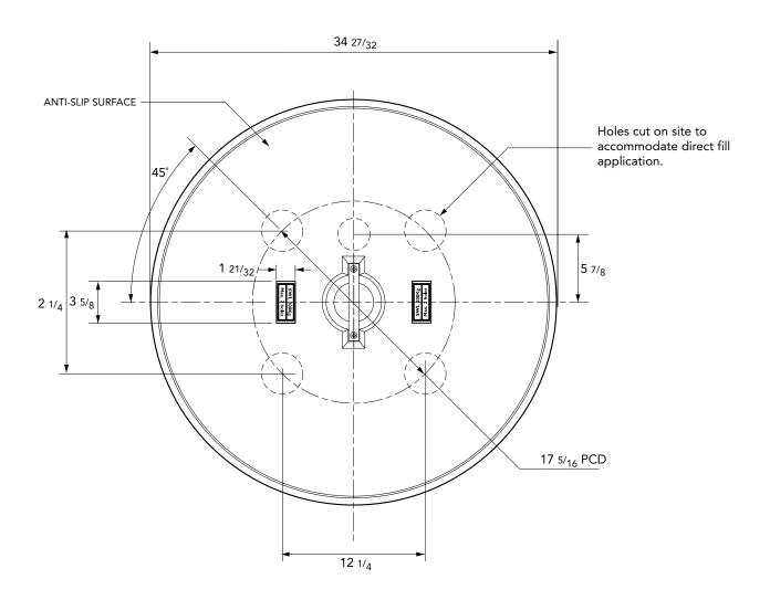
Hole configuration used for offset manual dipping.
