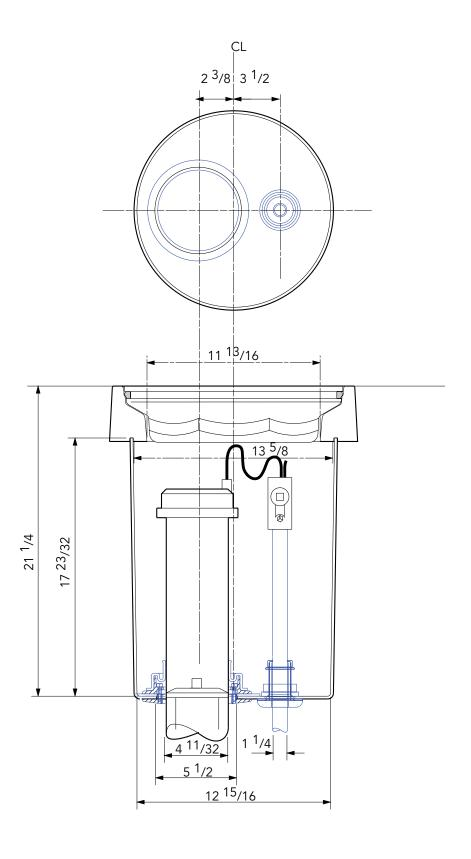
ATG Ground Box. 12" dia solid base sump with a 12" dia grey flat sealed cover and frame. One PSB/110 4 7/8" dia pipe sealkit. One PEC/32 1 1/4" dia conduit sealkit
