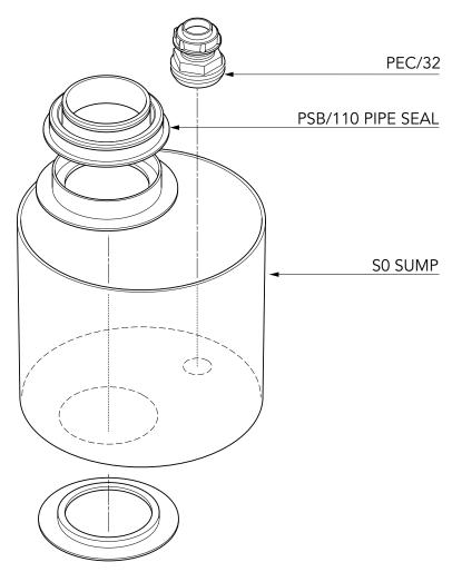
ATG Ground Box. 12" dia solid base sump with a 12" dia grey flat sealed cover and frame. One PSB/110 4 7/8" dia pipe sealkit. One PEC/32 1 1/4" dia conduit sealkit
