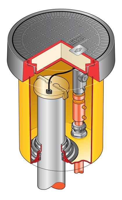
ATG Ground Box. 12" dia solid base sump with a 12" dia grey flat sealed cover and frame. One PSB/110 4 7/8" dia pipe sealkit. One PEC/32 1 1/4" dia conduit sealkit
