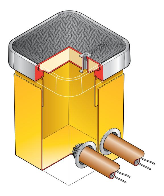
Electrical Drawpit 17 23/32" square x 23 5/8" GRP base chamber with a 8 1/4" deep skirt and square 17 23/32" at sealed cover.
