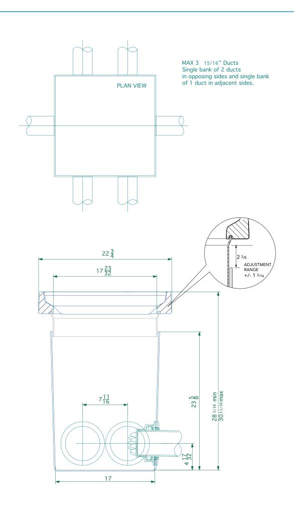
Electrical Drawpit 17 23/32" square x 23 5/8" GRP base chamber with a 8 1/4" deep skirt and square 17 23/32" at sealed cover.
