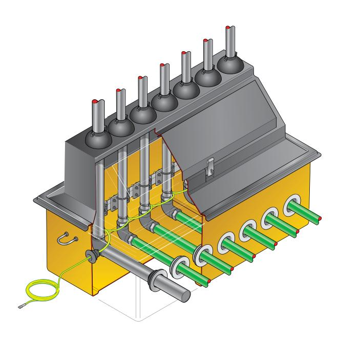
Vent pipe transition sump. 59" x 33" x 19" below ground solid base sump, with 18" high above ground sealed top with lockable hinged door. Includes pipework support rail and fixings. Order pipe entry boots PSB/63, PSB/90 PSB/63/VT, PSB/90/VT & vent riser mounting brackets MPK-VENT separately.
