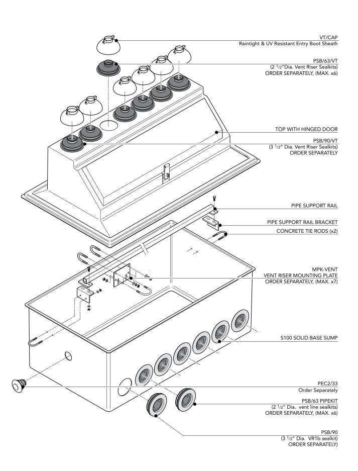
Vent pipe transition sump. 59" x 33" x 19" below ground solid base sump, with 18" high above ground sealed top with lockable hinged door. Includes pipework support rail and fixings. Order pipe entry boots PSB/63, PSB/90 PSB/63/VT, PSB/90/VT & vent riser mounting brackets MPK-VENT separately.
