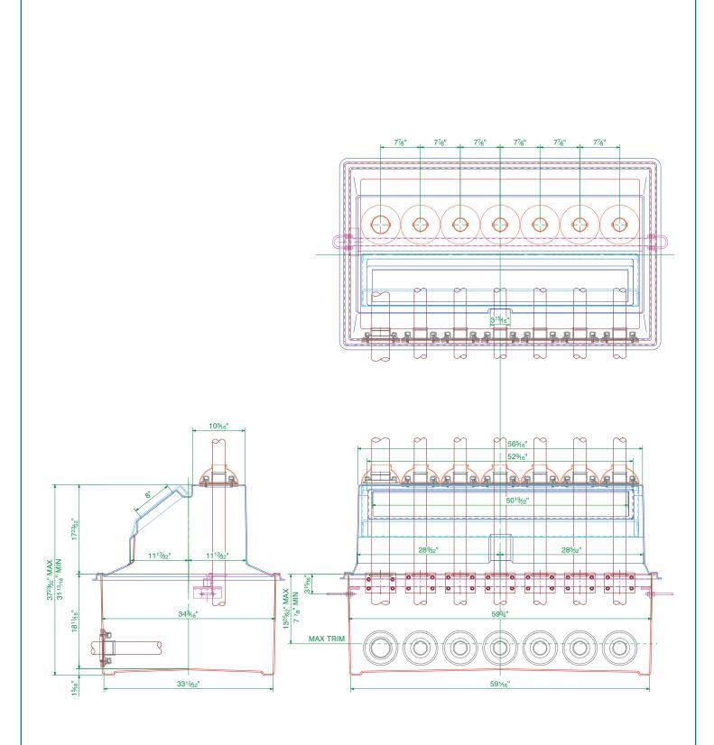
Vent pipe transition sump. 59" x 33" x 19" below ground solid base sump, with 18" high above ground sealed top with lockable hinged door. Includes pipework support rail and fixings. Order pipe entry boots PSB/63, PSB/90 PSB/63/VT, PSB/90/VT & vent riser mounting brackets MPK-VENT separately.
