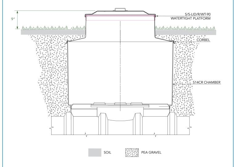
$52\ensuremath{^{"}}$  diameter sump with collar ring base, corbel and watertight platform for green areas.
