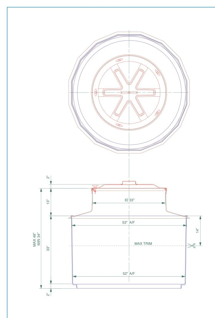
$52\ensuremath{^{\circ}}$  diameter sump with collar ring base, corbel and watertight platform for green areas.
