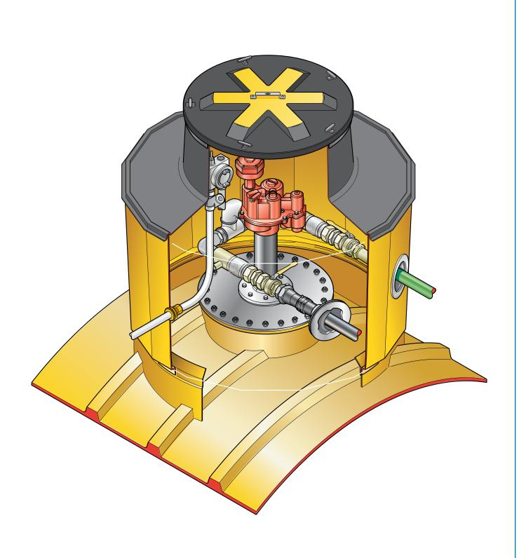
$52\ensuremath{^{\circ}}$  diameter sump with collar ring base, corbel and watertight platform for green areas.
