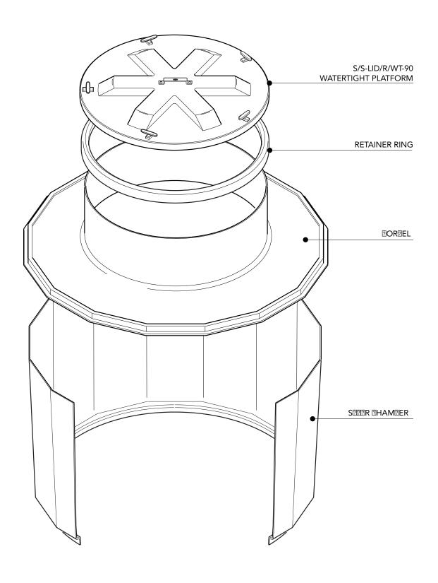
$52\ensuremath{^{\circ}}$  diameter sump with collar ring base, corbel and watertight platform for green areas.
