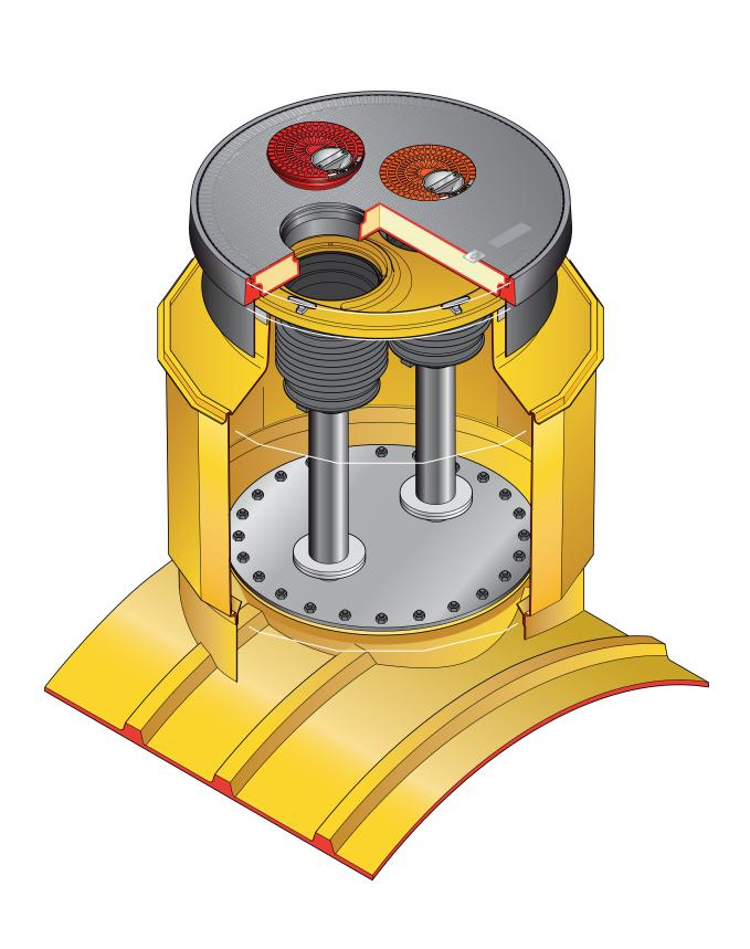
$1.4m\ diameter\ sump\ with\ collar\ ring\ base,\ corbel,\ skirt,\ spill\ container,\ round\ 1020mm\ flat\ sealed\ multiport\ cover\ with\ two\ port\ covers\ and\ frame.$
