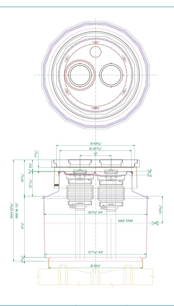
$1.4m\ diameter\ sump\ with\ collar\ ring\ base,\ corbel,\ skirt,\ spill\ container,\ round\ 1020mm\ flat\ sealed\ multiport\ cover\ with\ two\ port\ covers\ and\ frame.$
