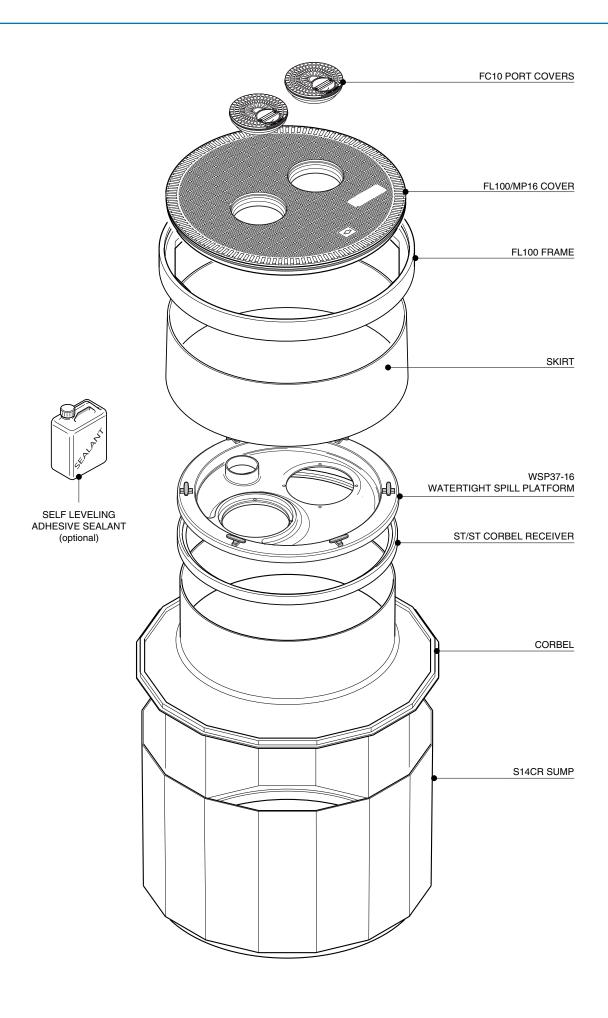
1.4m diameter sump with collar ring base, corbel, skirt, spill container, round 1020mm flat sealed multiport cover with two port covers and frame.
