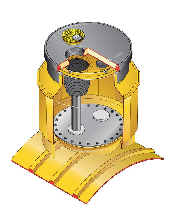
52" diameter x 33" deep sump base to fit 48" tank collar ring, corbel and watertight spill platform for a single 5-gallon spill bucket. 40" diameter offset fill cover, frame and skirt.
