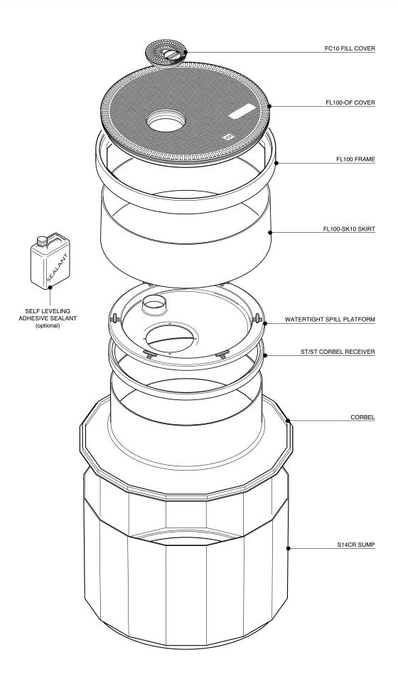
52" diameter x 33" deep sump base to fit 48" tank collar ring, corbel and watertight spill platform for a single 5-gallon spill bucket. 40" diameter offset fill cover, frame and skirt.
