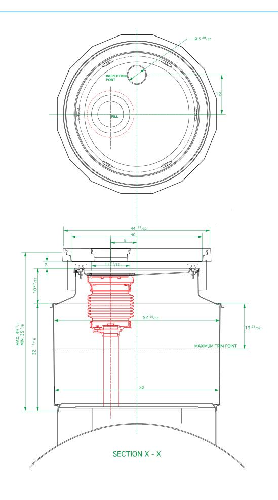
52" diameter x 33" deep sump base to fit 48" tank collar ring, corbel and watertight spill platform for a single 5-gallon spill bucket. 40" diameter offset fill cover, frame and skirt.
