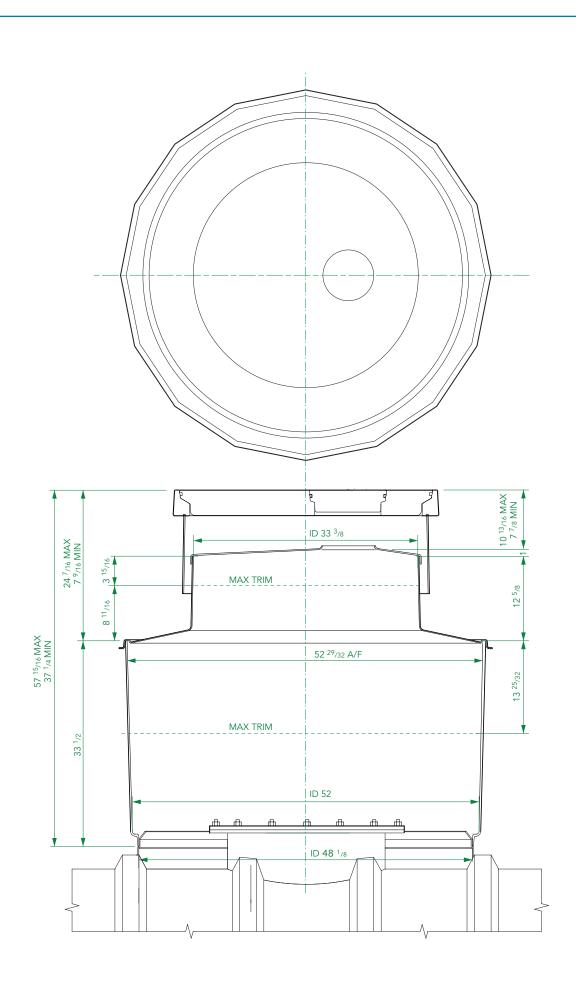
54" diameter sump to fit 48" collar ring, with corbel, internal lid, adjustable skirt and round 36" flat sealed cover, corbel/skirt sealkit with condensation bottle and fixing kit.
