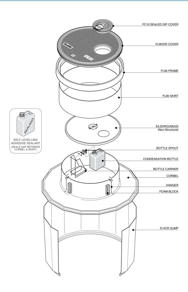
54" diameter sump to fit 48" collar ring, with corbel, internal lid, adjustable skirt and round 36" flat sealed cover, corbel/skirt sealkit with condensation bottle and fixing kit.
