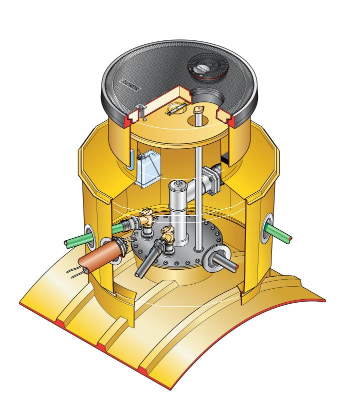
$54^{\circ}$  diameter sump to fit  $48^{\circ}$  collar ring, with corbel, internal lid, adjustable skirt and round  $36^{\circ}$  flat sealed cover, corbel/skirt sealkit with condensation bottle and fixing kit.
