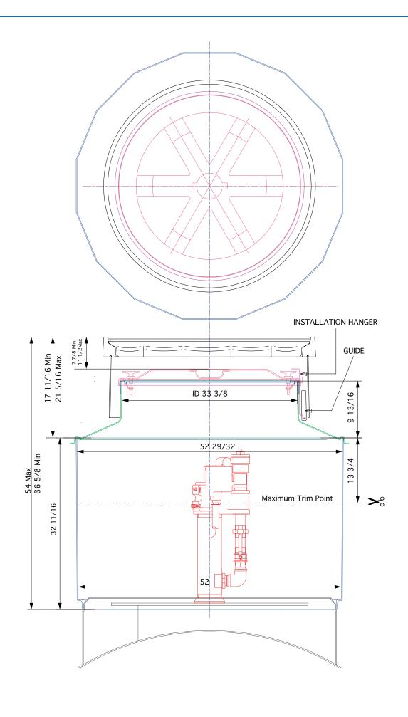
Watertight FRP sump to fit 48" tank collar, FRP corbel, watertight inner sump lid and 36" diameter, watertight, flat sealed manhole cover.
