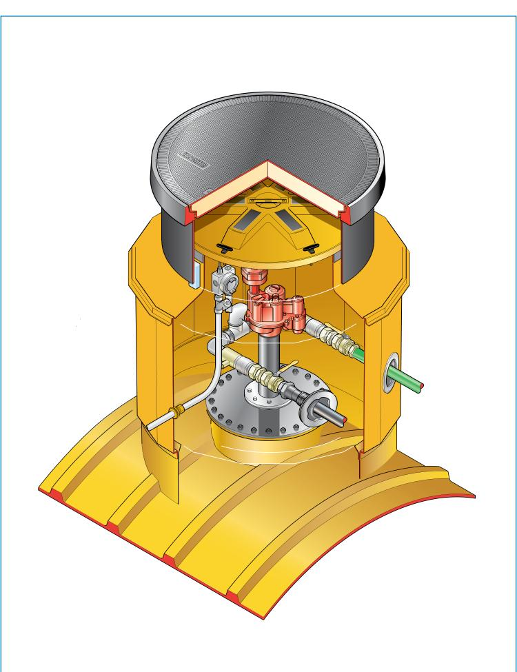
Watertight FRP sump to fit 48" tank collar, FRP corbel, watertight inner sump lid and 36" diameter, watertight, flat sealed manhole cover.
