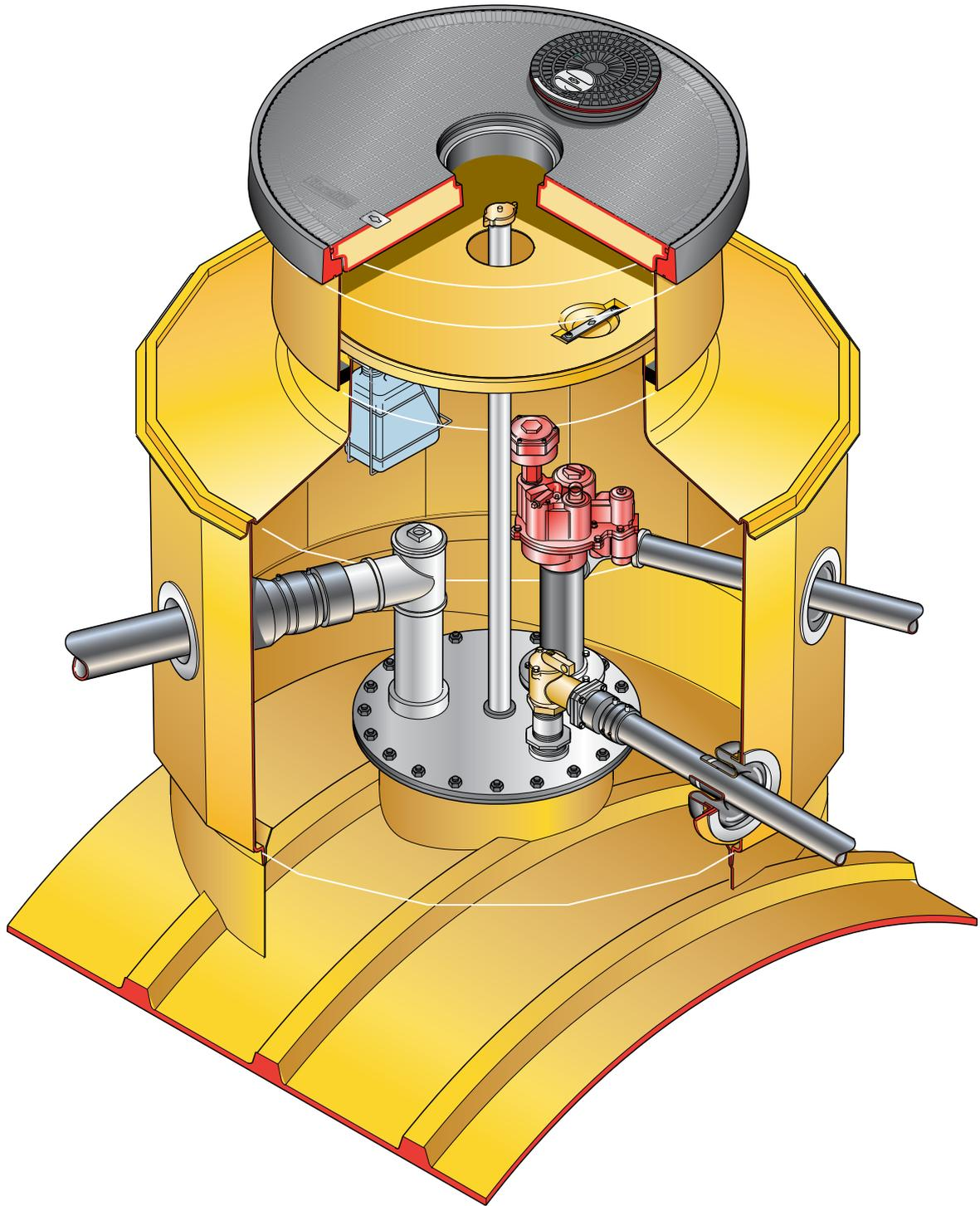
57" dia. FRP sump with 54" tank collar ring connection, corbel, skirt, internal lid, 36" dia. flat sealed cover with central manual dip cover and frame.
