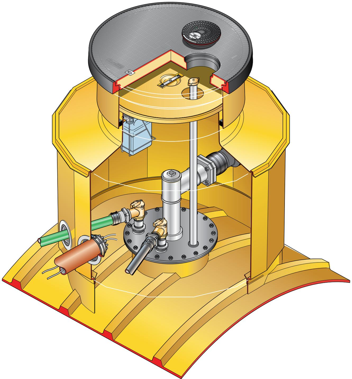
57" dia. FRP sump with 54" tank collar ring connection, corbel, skirt, internal lid, 36" dia. flat sealed cover with offset manual dip cover and frame.
