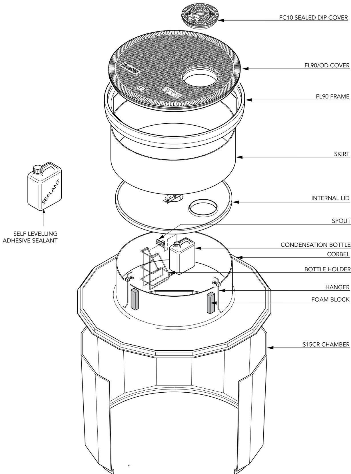
57" dia. FRP sump with 54" tank collar ring connection, corbel, skirt, internal lid, 36" dia. flat sealed cover with offset manual dip cover and frame.
