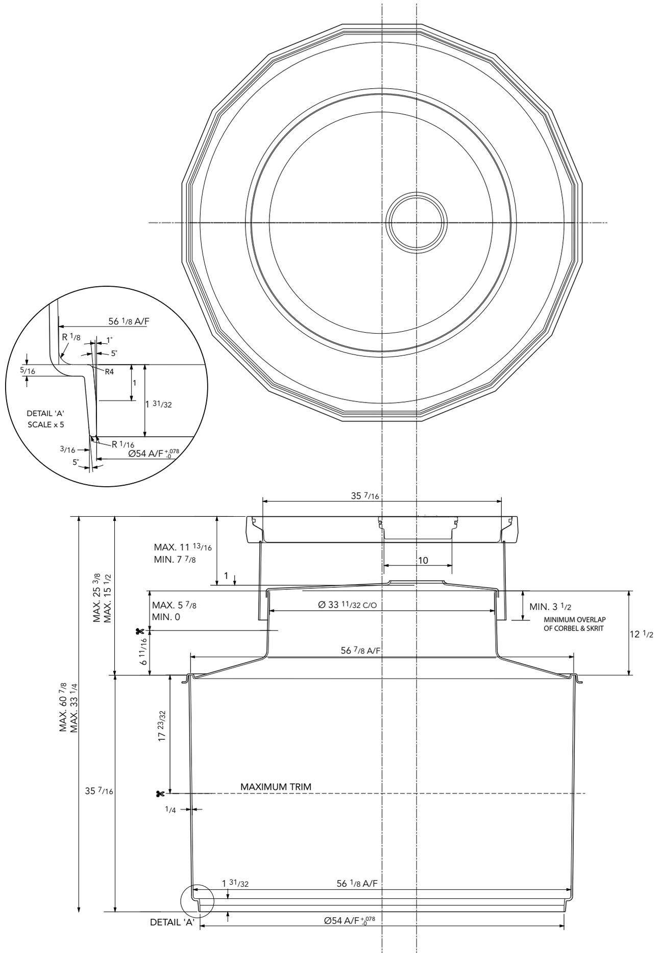
57" dia. FRP sump with 54" tank collar ring connection, corbel, skirt, internal lid, 36" dia. flat sealed cover with offset manual dip cover and frame.
