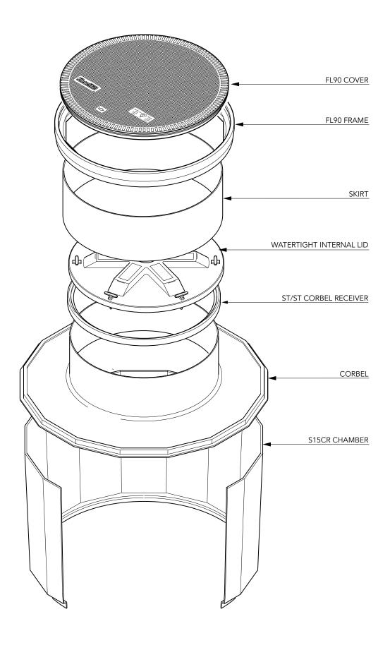
$57^{\circ}$  dia. FRP sump with  $54^{\circ}$  tank collar ring connection, corbel, skirt, watertight internal lid,  $36^{\circ}$  dia. flat cover and composite frame.
