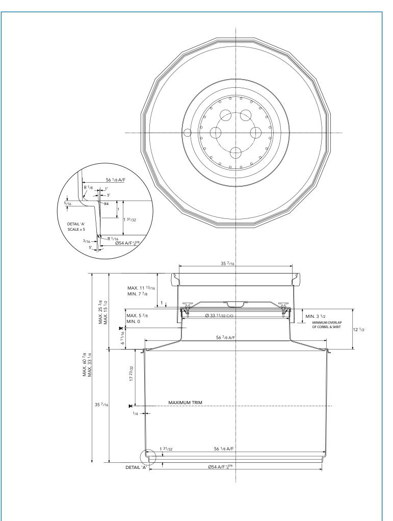
$57^{\circ}$  dia. FRP sump with  $54^{\circ}$  tank collar ring connection, corbel, skirt, watertight internal lid,  $36^{\circ}$  dia. flat cover and composite frame.
