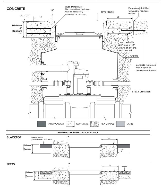
57" dia. FRP sump with 54" tank collar ring connection, corbel, skirt, watertight internal lid, 36" dia. flat cover and composite frame.
